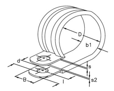
$\begin{array}{lll} b1 & = 15.0 \\ d & = 6.4 \\ Diameter D = 10 \\ I & = 6 \\ s & = 0.8 \\ s2 & = 1.2 \\ Width B & = 12 \\ \end{array}$
